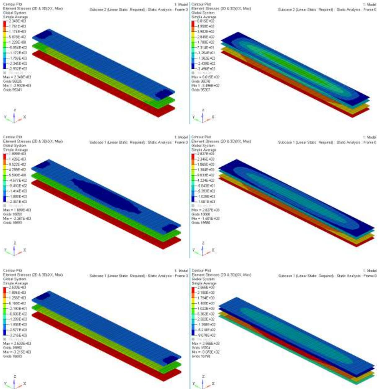
**Figure 8.16: FML flexure test verification, X-Stress (MPa) fringe in AL 1100 (left) and Composites (right); FML01 (top), FML02 (middle) and FML03 (bottom)**
