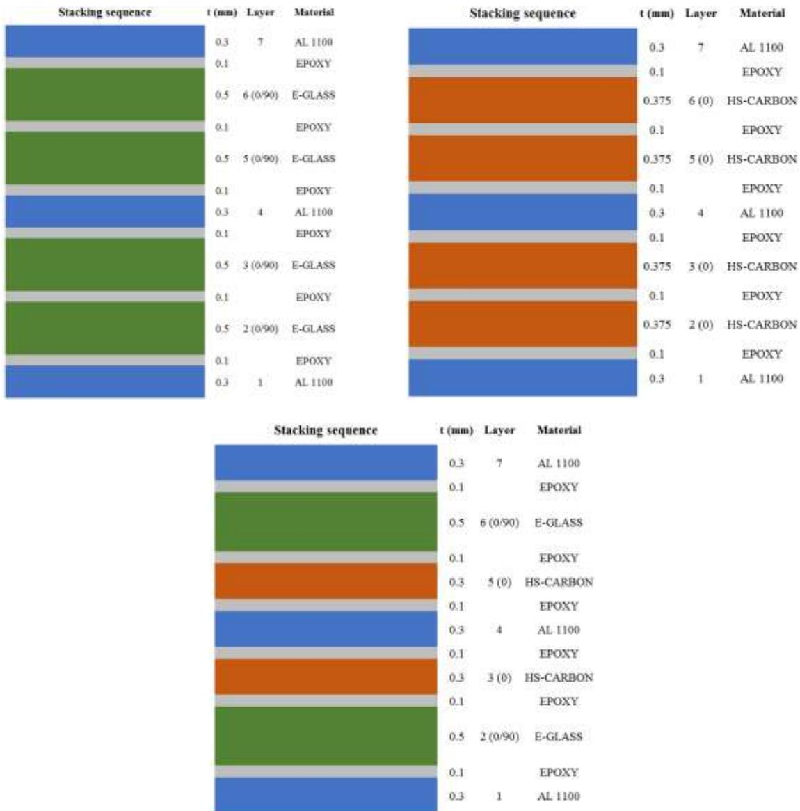
**Figure 8.1: Stacking sequence for FEA of FML01 (top left), FML02 (top right) and FM03 (bottom)**
