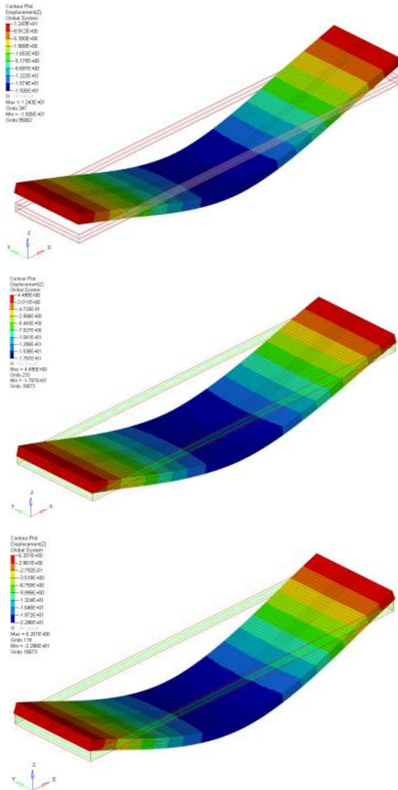
**Figure 8.15: FML flexure test verification, Deformation with Z-Displacement (mm) fringe; FML01 (top), FML02 (middle) and FML03 (bottom)**
