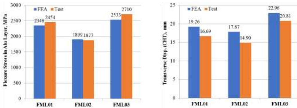
**Figure 8.18: FML flexure test verification – Test vs. FEA**
