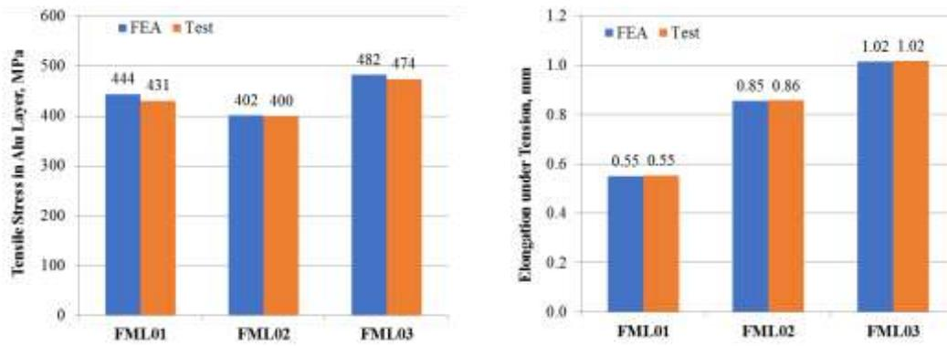
**Figure 8.17: FML tensile test verification – Test vs. FEA**
