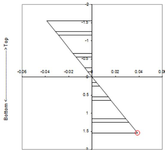
**Figure 8.14: Flexural strain variation for three point bending of FML composite specimen, (e.g. FML03)**
