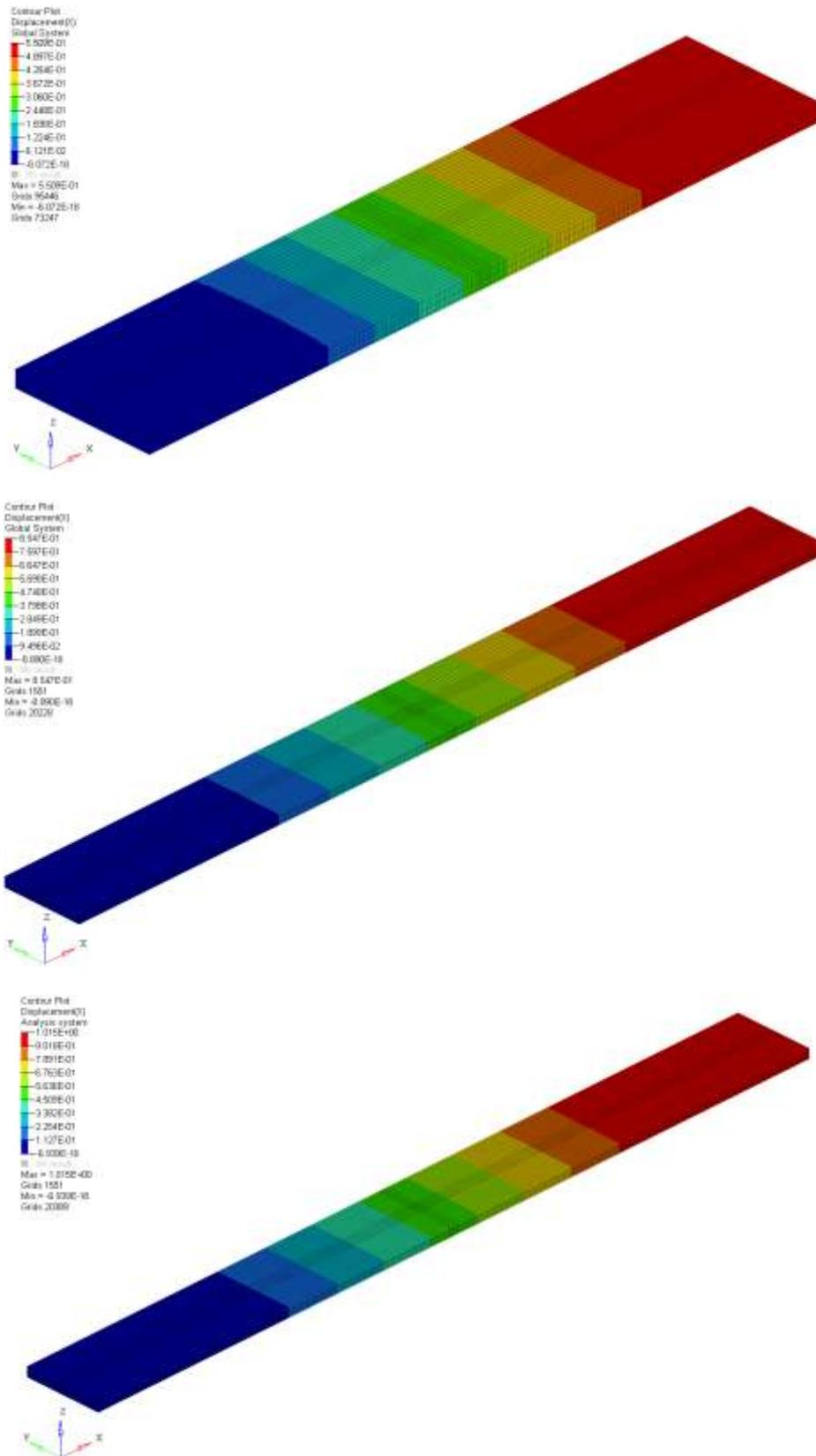
**Figure 8.12: FML tensile test verification, X-Displacement (mm) fringe; FML01 (top), FML02 (middle) and FML03 (bottom)**
