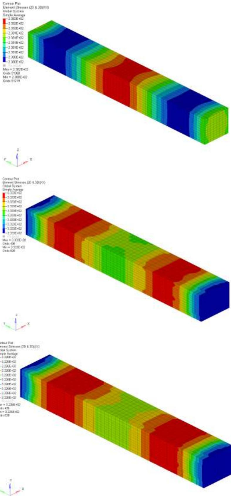
**Figure 8.9: Tensile test BC validation using neat resin property, X-Stress (MPa) fringe; FML01 (top), FML02 (middle) and FML03 (bottom)**
