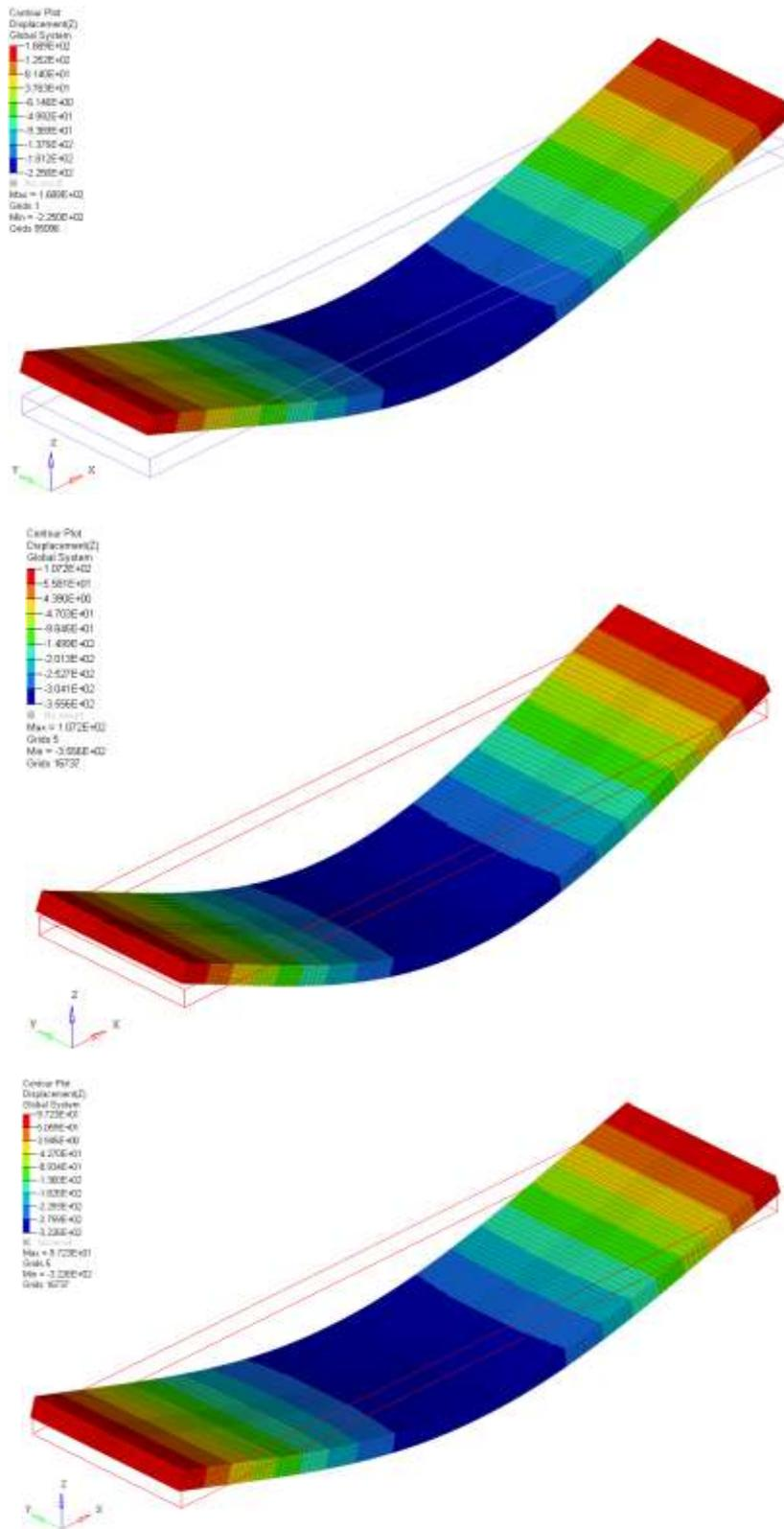
**Figure 8.10: Flexure test BC validation using neat resin property, Deformation with Z-Displacement (mm) fringe; FML01 (top), FML02 (middle) and FML03 (bottom)**
