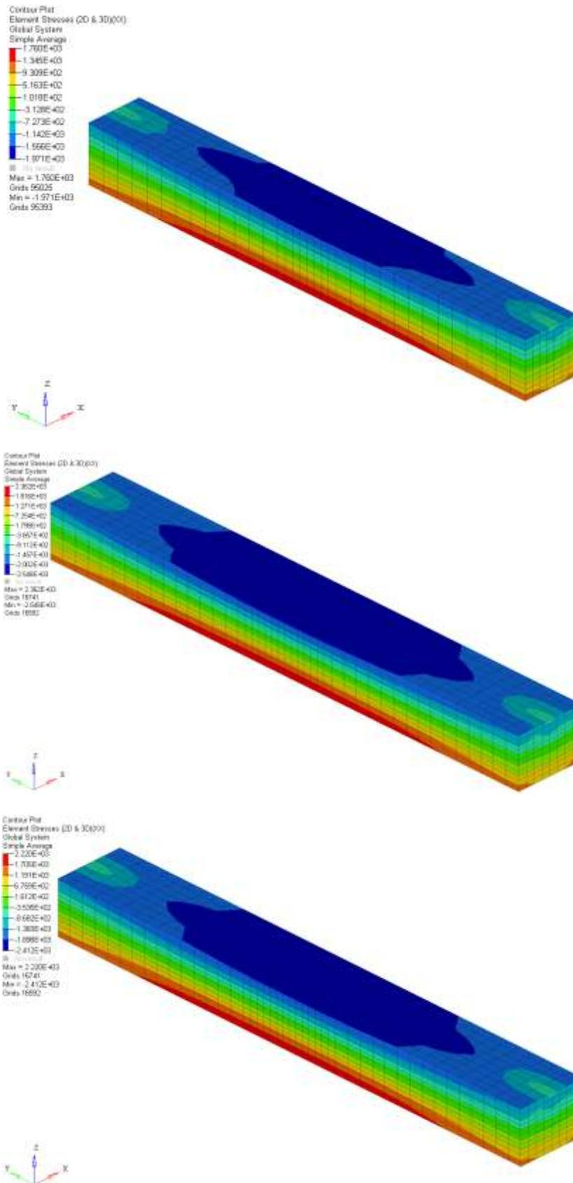
**Figure 8.11: Flexure test BC validation using neat resin property, X-Stress (MPa) fringe; FML01 (top), FML02 (middle) and FML03 (bottom)**
