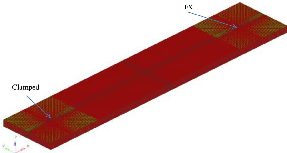
**Figure 8.6: Boundary conditions and loading for tensile test (e.g. M111)**
