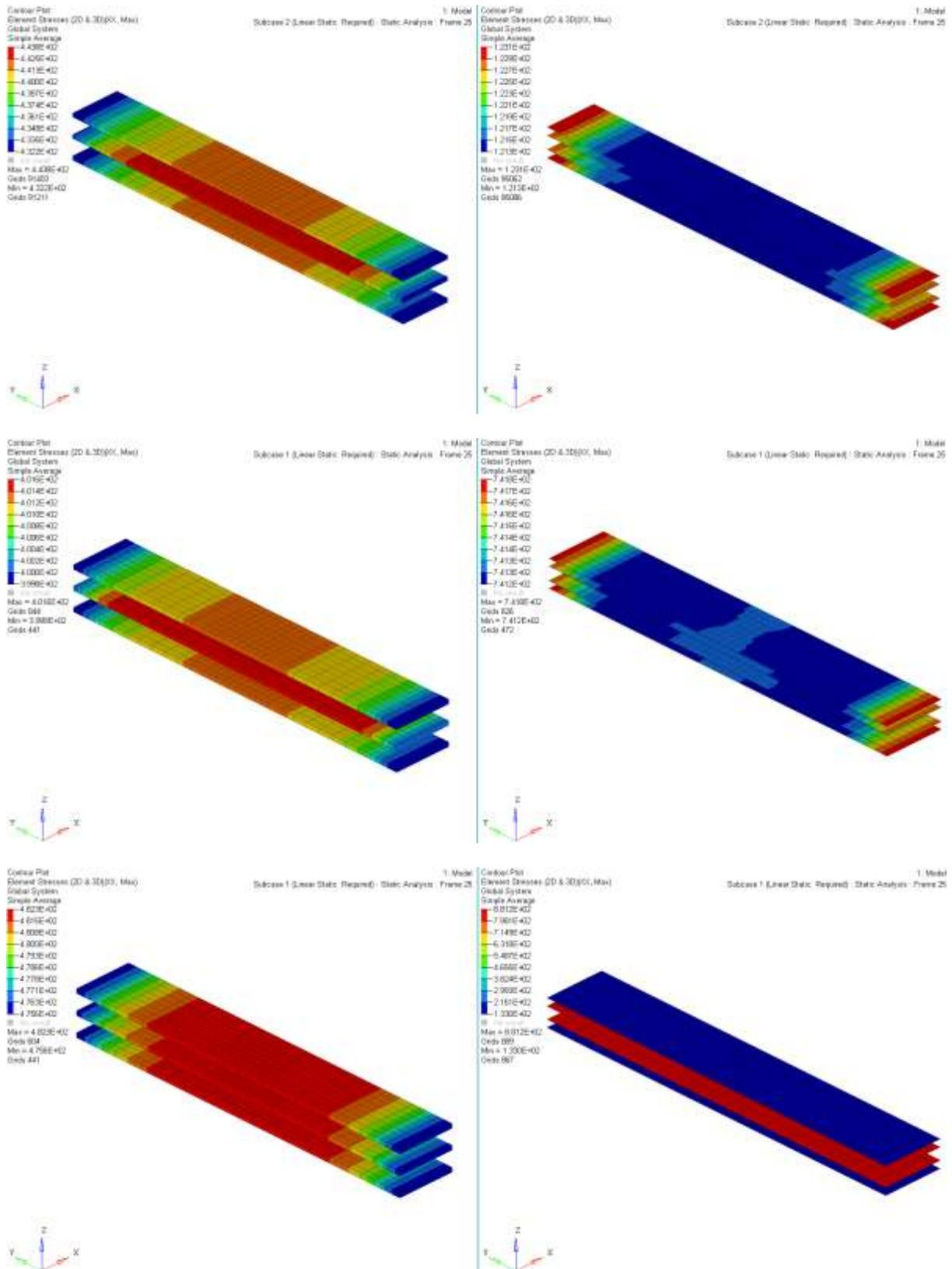
**Figure 8.13: FML tensile test verification, X-Stress (MPa) fringe in AL 1100 (left) and Composites (right); FML01 (top), FML02 (middle) and FML03 (bottom)**
