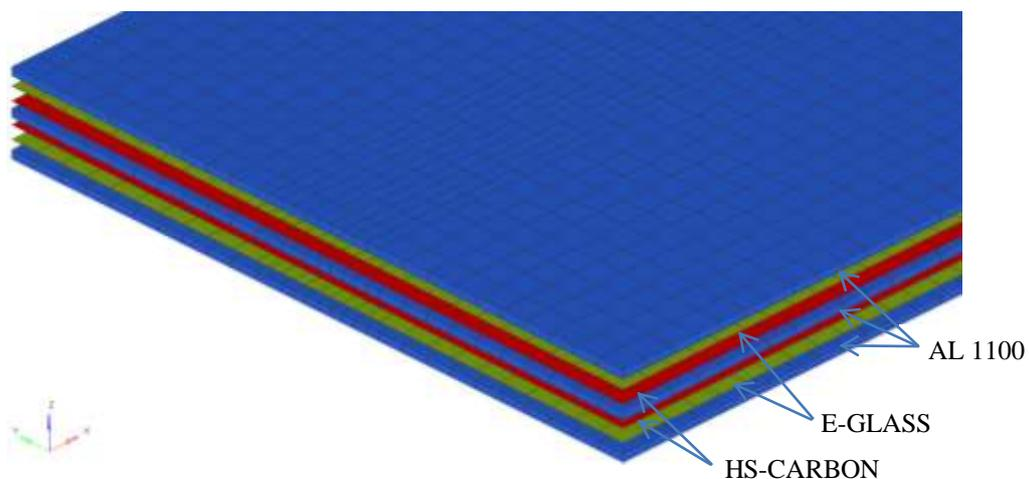
**Figure 8.3: FE mesh of FML reinforcement layers (resin mesh not shown)**
