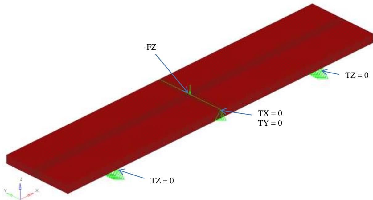
**Figure 8.7: Boundary conditions and loading for flexure test (e.g. M112)**
