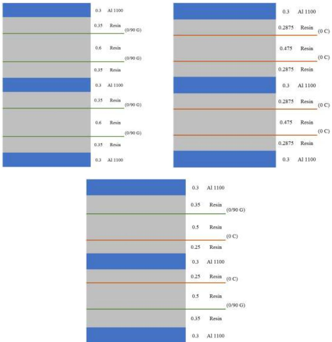
**Figure 8.2: Idealisation of composite and metallic plies for FEA of FML01 (top left), FML02 (top right) and FML03 (bottom)**
