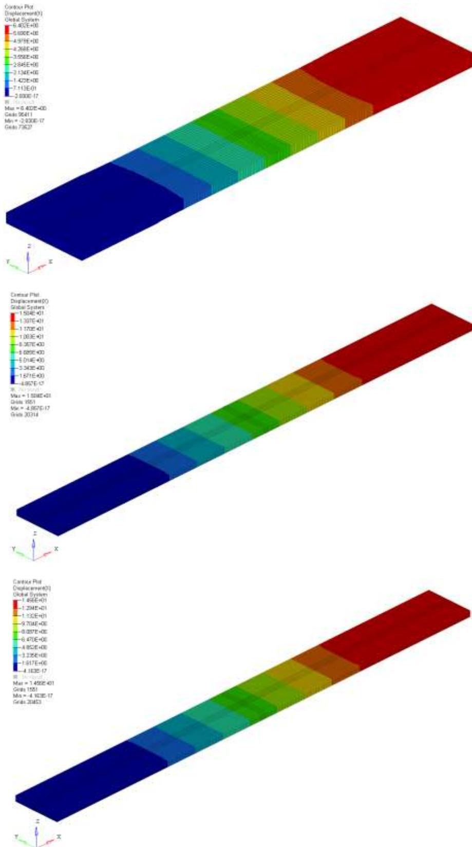
**Figure 8.8: Tensile test BC validation using neat resin property, X-Displacement (mm) fringe; FML01 (top), FML02 (middle) and FML03 (bottom)**
