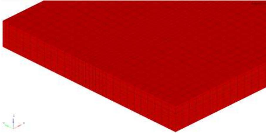
**Figure 8.4: FE mesh refinement at edge of the specimen**
