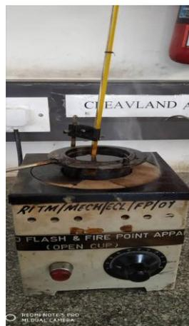
Fig. 2: Flash point test
