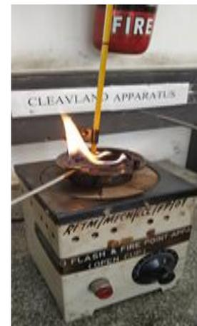
Fig. 3: Fire point test
