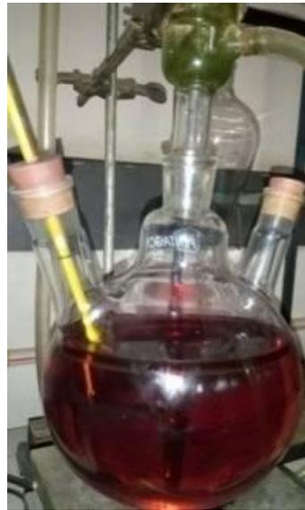
Fig. 1: Batch reactor for transesterification
