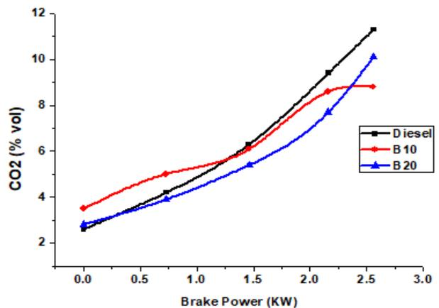
Fig. 9: CO<sub>2</sub> (hybrid biodiesel) vs. BP
