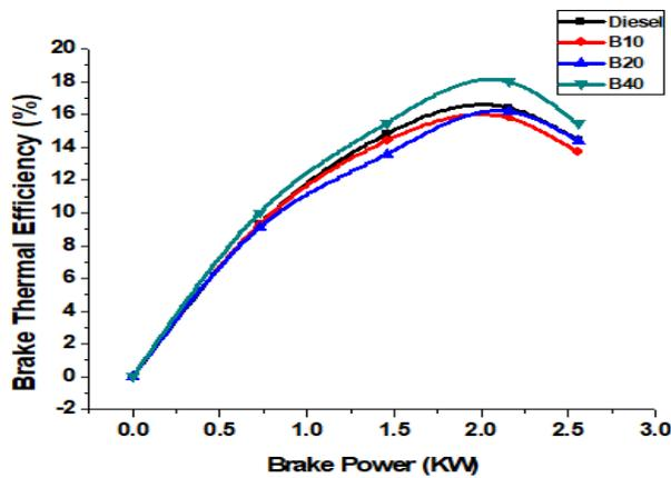
Fig. 5: BTE (hybrid biodiesel) vs. BP
