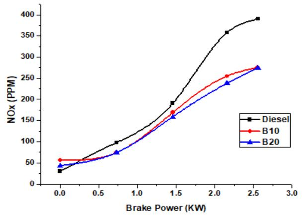
Fig. 7: NO<sub>x</sub> (hybrid biodiesel) vs. BP
