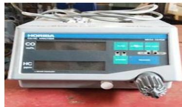
**Fig. 2: Exhaust gas analyser**
