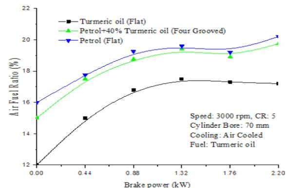
Fig. 8: Effects of BP on air fuel ratio – Turmeric oil B40 blend
