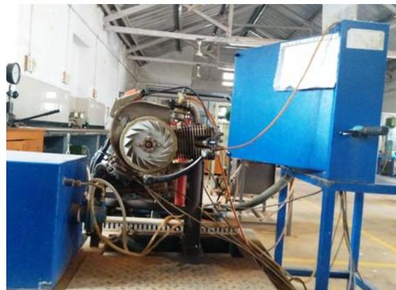
**Fig. 1: Petrol engine test rig**
