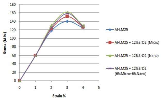
**Fig. 2: Stress strain diagram**
