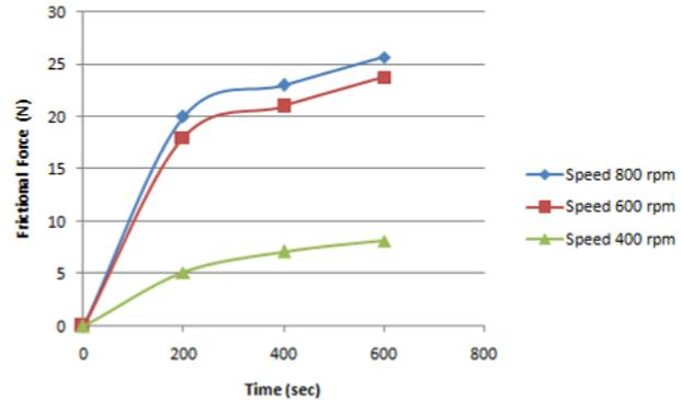
**Fig. 4(a): Friction force vs. Time - Al-LM25 + 12%ZrO<sub>2</sub> (Micro)**
