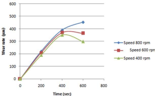
**Fig. 3(b): Wear rate vs. Time - Al-LM25 + 12%ZrO<sub>2</sub> (Nano)**
