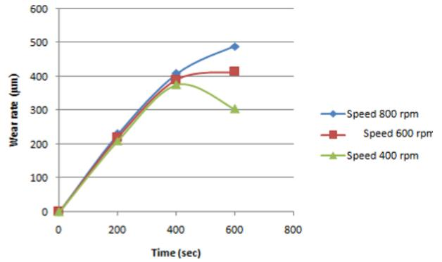
**Fig. 3(c): Wear rate vs. Time - Al-LM25 + 6% ZrO<sub>2</sub>Micro+6% ZrO<sub>2</sub>Nano**
