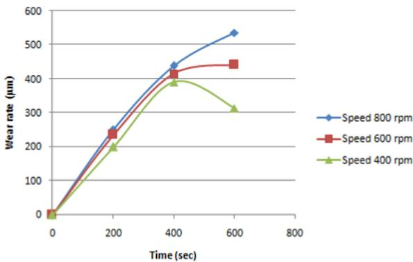
**Fig. 3(a): Wear rate vs. Time - Al-LM25 + 12%ZrO<sub>2</sub> (Micro)**
