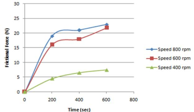
**Fig. 4(c): Friction force vs. Time - Al-LM25 + 6% ZrO<sub>2</sub>Micro+6% ZrO<sub>2</sub>Nano**
