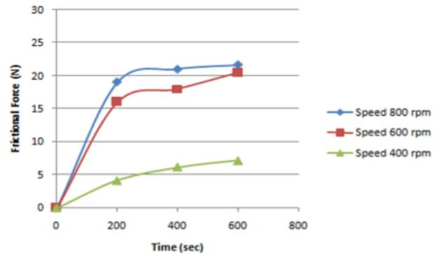
**Fig. 4(b): Friction force vs. Time - Al-LM25 + 12%ZrO<sub>2</sub> (Nano)**
