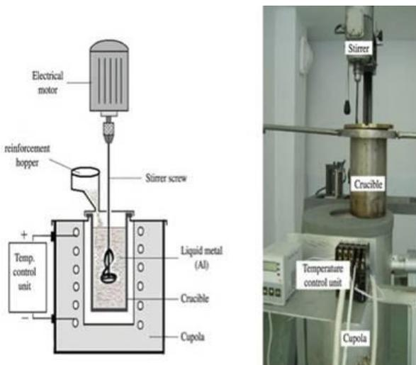
**Fig. 1: Stir casting**
