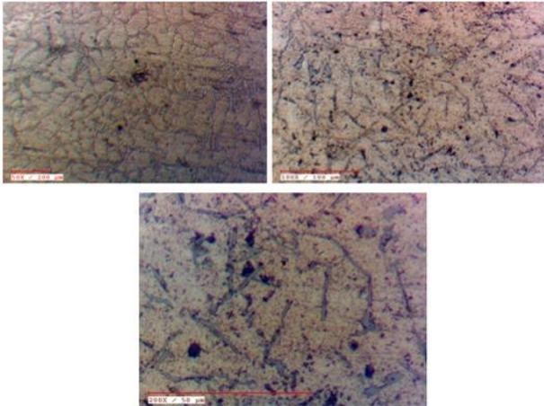
Fig. 5: Optical micrographs of Al-LM25 + 12%ZrO<sub>2</sub> (micro)
