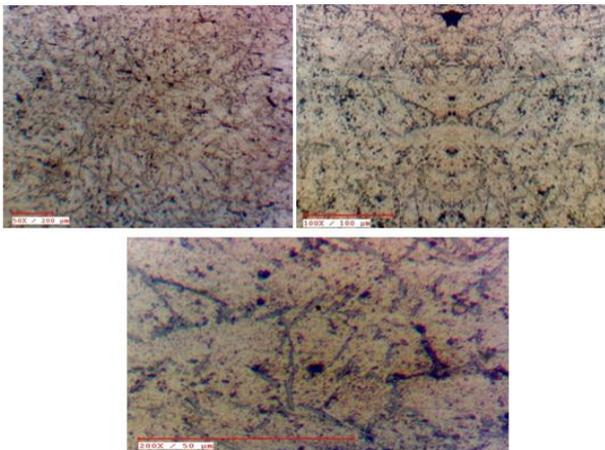
Fig. 6: Optical micrographs of Al-LM25 + 12%ZrO<sub>2</sub> (nano)
