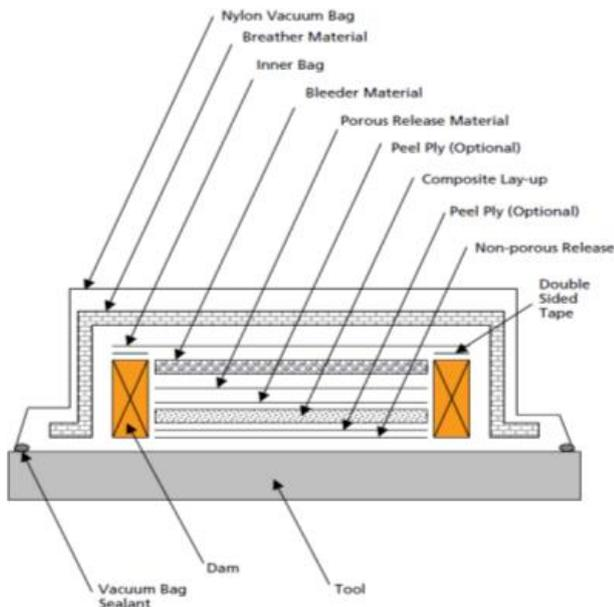
Fig. 5: Composite part layup process
