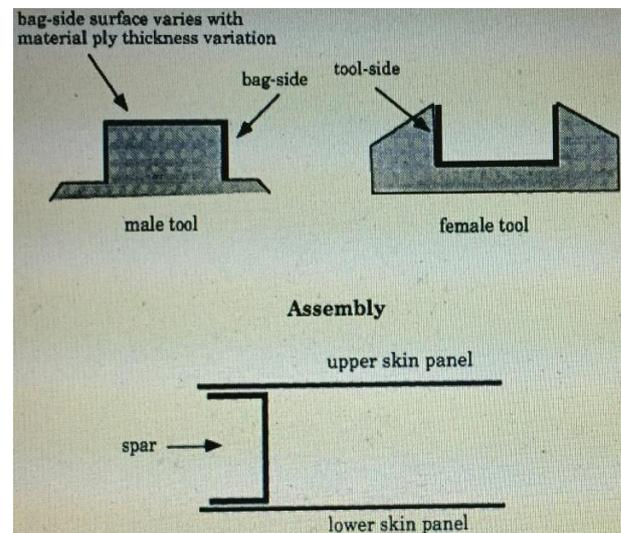
Fig. 2: Male vs. Female tool and spar assembly process
