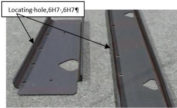
Fig. 3: Composite spar manufactured with newly designed tool
