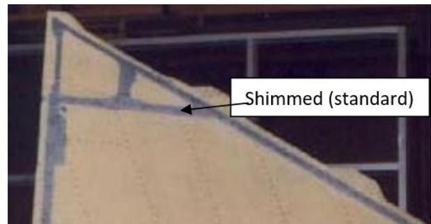
Fig. 11: Shimming process carried out on composite skin with new mould tool using research experiment
