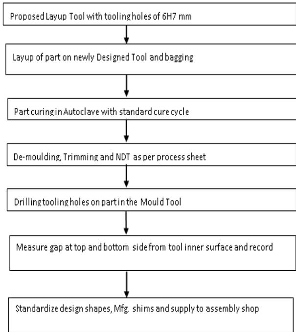
Fig. 9: Flow chart of newly designed composite part manufacturing
