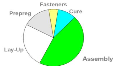
Fig. 1: Relative cost distribution of Tejas composite wing assembly
