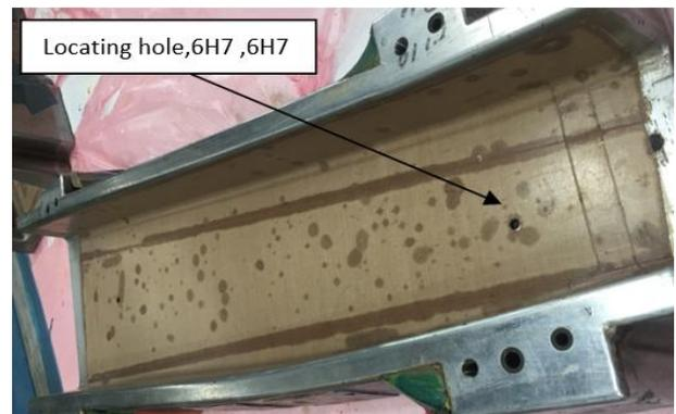
Fig. 7: New mould tool with 6H7 mm tooling hole
