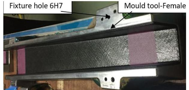
Fig. 6: Composite part lay-up in newly designed tool
