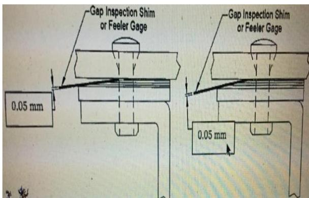
Fig. 10: Gap measurement method at spar to skin interface
