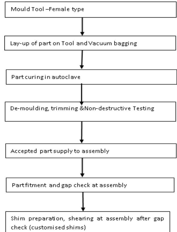
Fig. 8: Flow chart of existing composite part manufacturing
