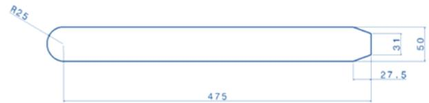
Fig. 2: Boat tail base configuration
