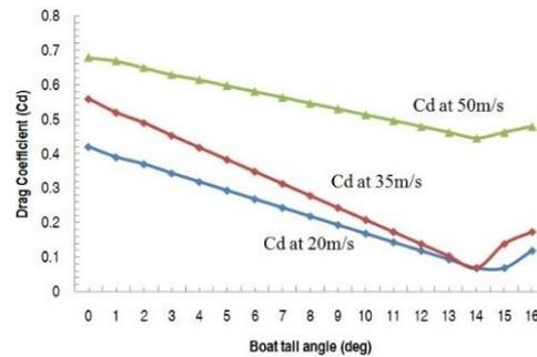
Fig. 8: Effect of  $C_d$  on boat tail angle at different velocities
