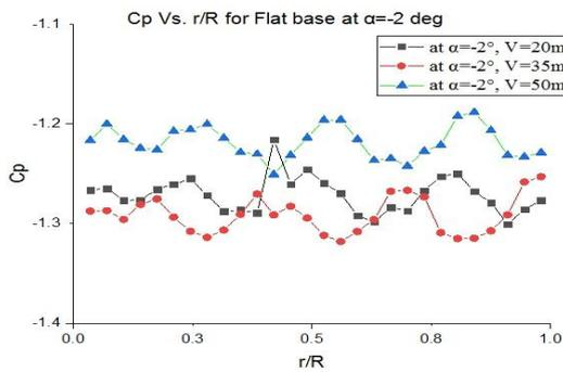
Fig. 6:  $C_p$  vs.  $r/R$  for boat tail base at  $\alpha = -2^\circ$
