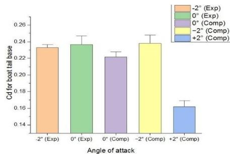
Fig. 9:  $C_d$  vs. AoA for boat tail base at 20m/s
