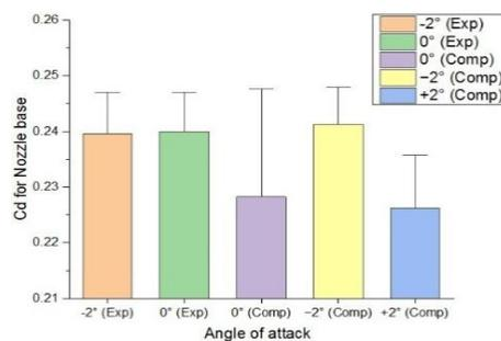
Fig. 10:  $C_d$  vs. AoA for boat tail base at 35m/s
