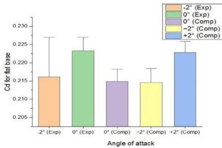
Fig. 11: Cd vs. AoA for boat tail base at 50m/s
