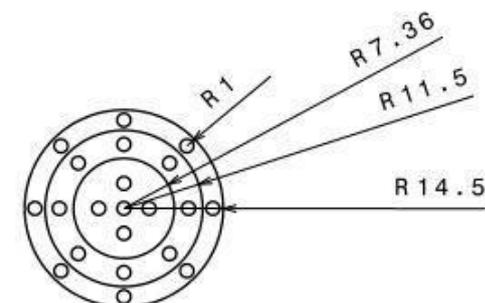
Fig. 4: Ports distribution in boat tail base
