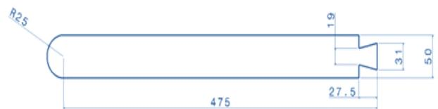
Fig. 3: Nozzle base configuration
