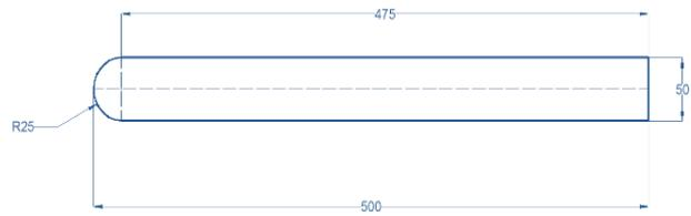
Fig. 1: Base line configuration
