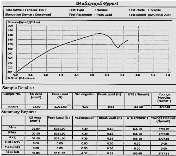
Fig. 15: Tensile stress-strain plot for EPWM12 + 1.5% GO laminate
