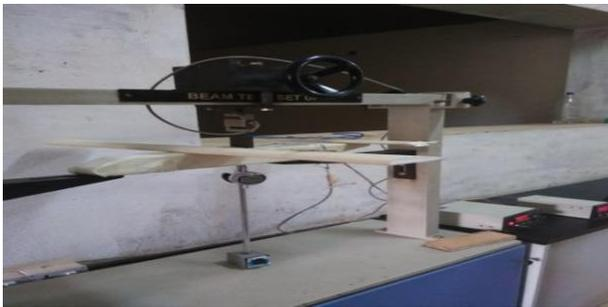
Fig. 14: Fuselage bending test
