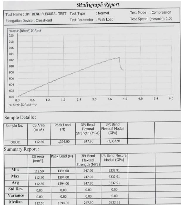
Fig. 10: Flexural stress-strain plot for EPWM12 + 1.5% GO laminate
