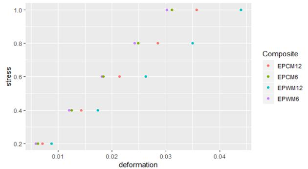
Fig. 11: Comparison of stress-deformation for four composites under three-point bend flexural test
