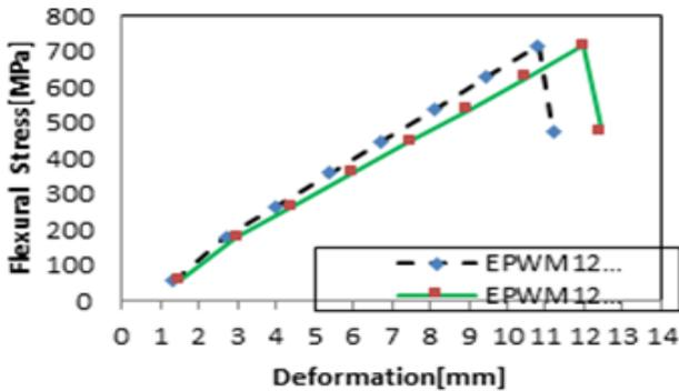
Fig. 15: Flexural stress vs. Deformation from bending test for wing (continuous line) and fuselage (dotted line)
