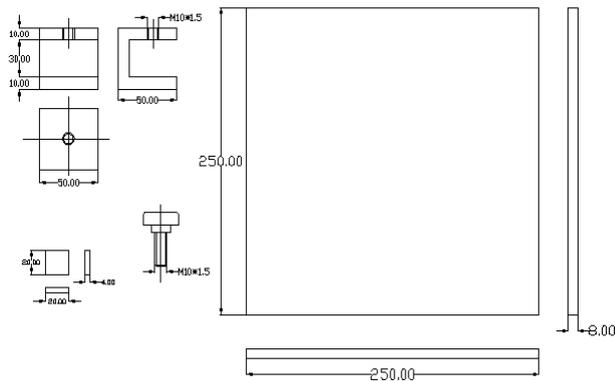
**Fig. 1: Drawing for the fabrication mould**
