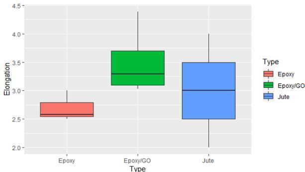
Fig. 9: % Elongation results from tensile test
