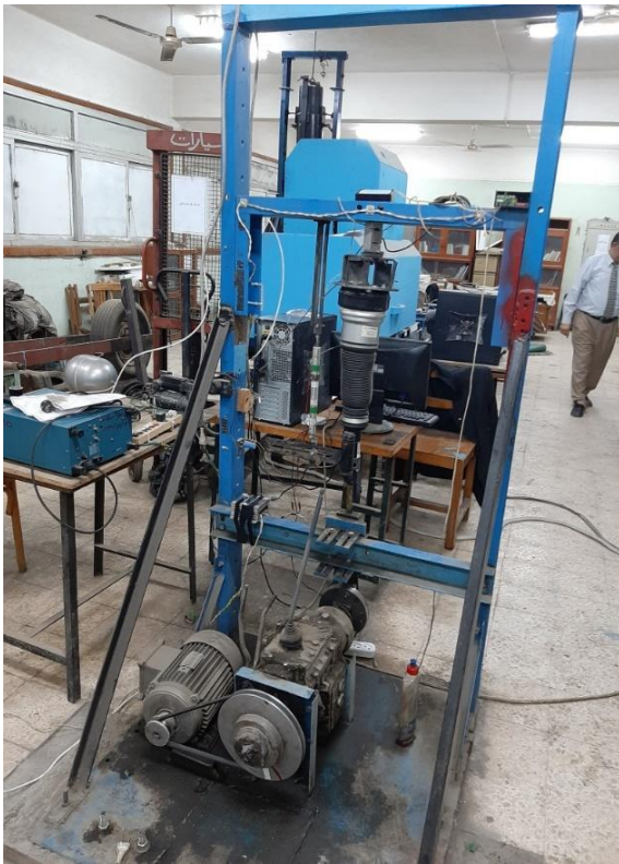
Fig. 1: Damper characteristics test rig
