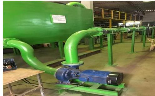
Fig. 2: Test set up for butterfly valve with double offset disc
