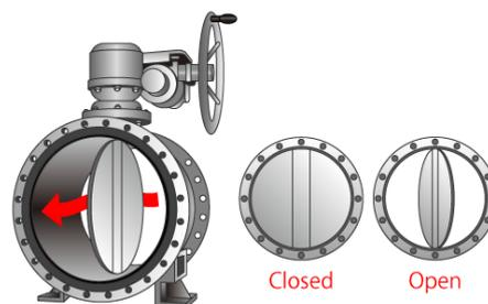
Fig. 1: Butterfly valve, closed and open position
