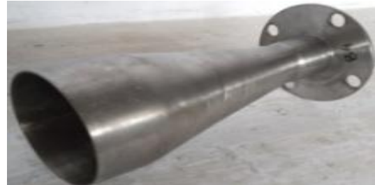
Fig. 11: Bell shaped nozzle configuration - 4
