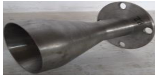
Fig. 9: Bell shaped nozzle configuration - 2
