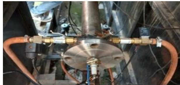
Fig. 3: Fuel injection/ air delivery system
