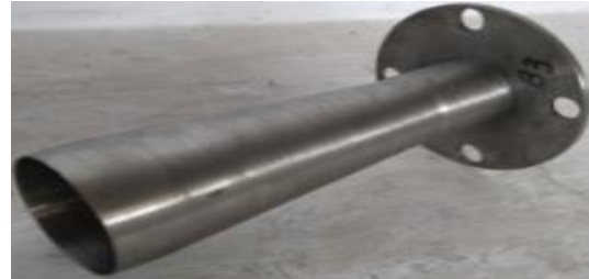
Fig. 10: Bell shaped nozzle configuration - 3
