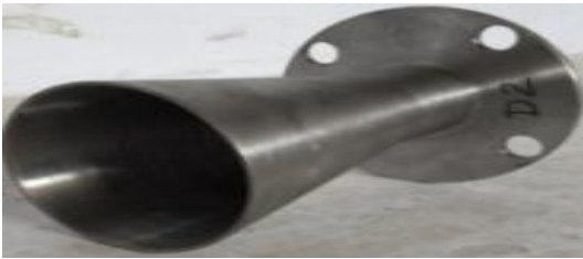
Fig. 5: Divergent nozzle configuration - 2
