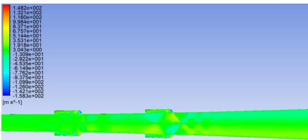
Fig. 12: Velocity contour for dual cavity case 3
