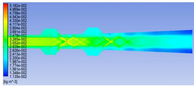
Fig. 28: Density contour for case 5
