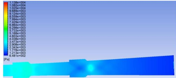
Fig. 5: Pressure contour for dual cavity case 2
