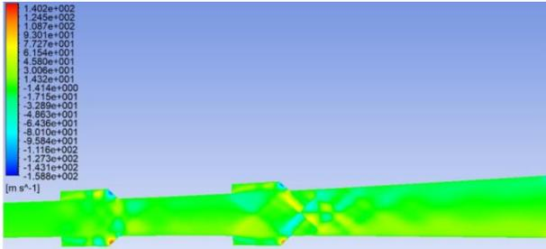
Fig. 10: Velocity contour for dual cavity case 1
