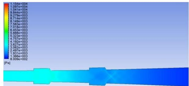
Fig. 6: Pressure contour for dual cavity case 3
