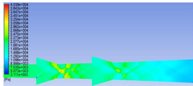
Fig. 7: Pressure contour for dual cavity case 4
