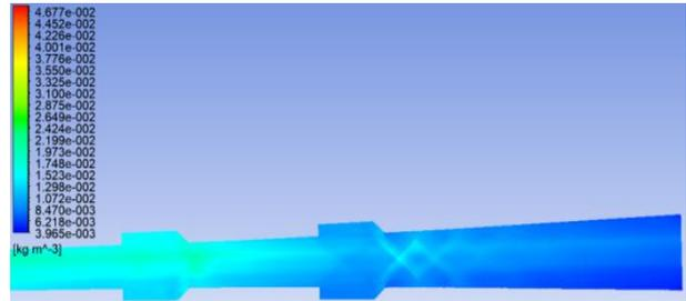
Fig. 24: Density contour for case 1
