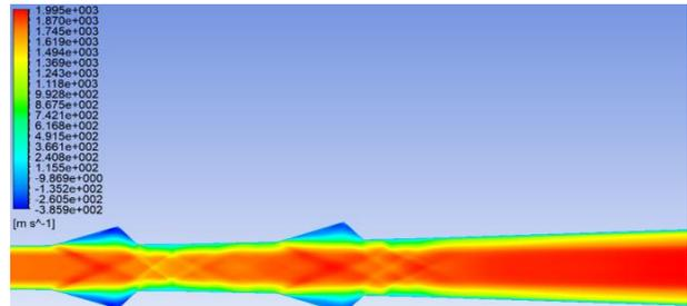
Fig. 16: Velocity contour for dual cavity case 6
