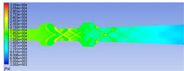
Fig. 8: Pressure contour for dual cavity case 5
