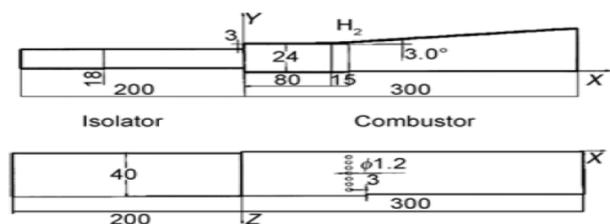
Fig. 1: Combustor rig configuration
