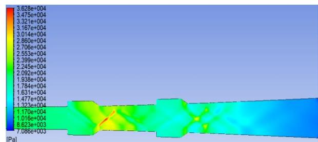
Fig. 9: Pressure contour for dual cavity case 6
