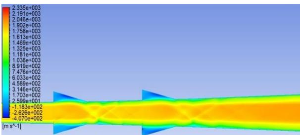
Fig. 13: Velocity contour for dual cavity case 4
