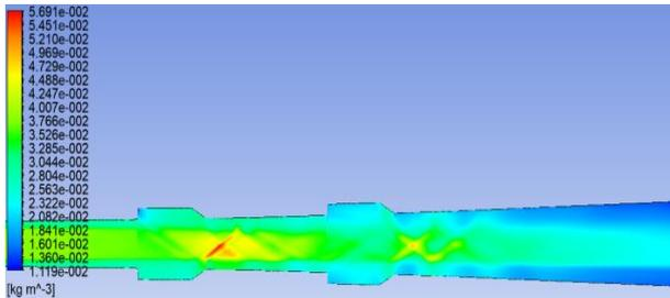
Fig. 29: Density contour for case 6
