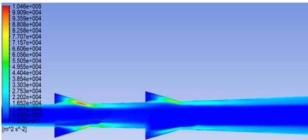
Fig. 20: Turbulence kinetic energy for case 4
