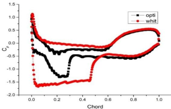
Fig. 12: Cp contour - Whitcomb IL airfoil vs. Optimized airfoil
