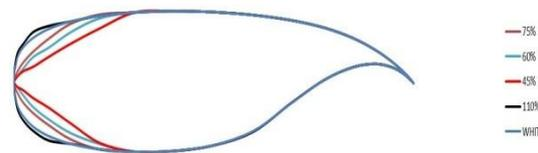
**Fig. 1: Different thickness edge thickness of Whitcomb airfoil**
