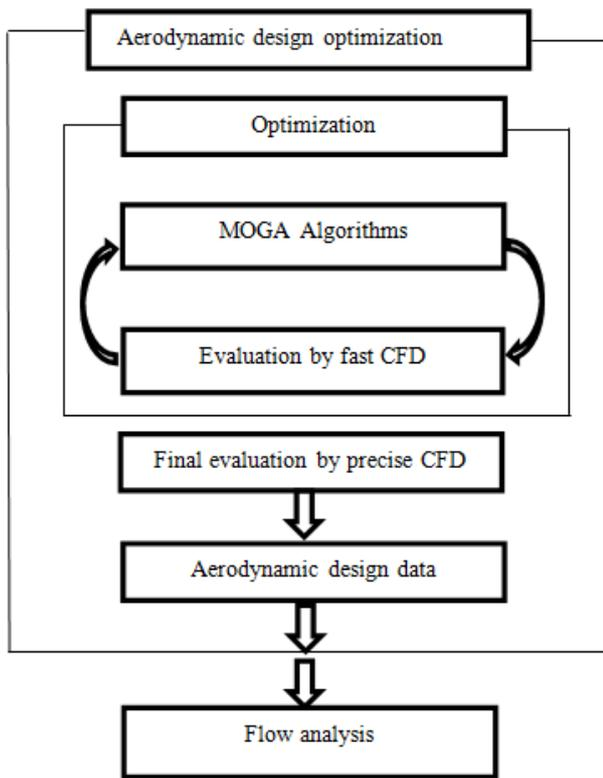
Fig. 4: Diagram of information flow in MOGA
