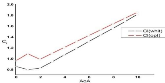
Fig. 8:  $C_l$  vs. AoA for Whitcomb IL and optimized airfoil
