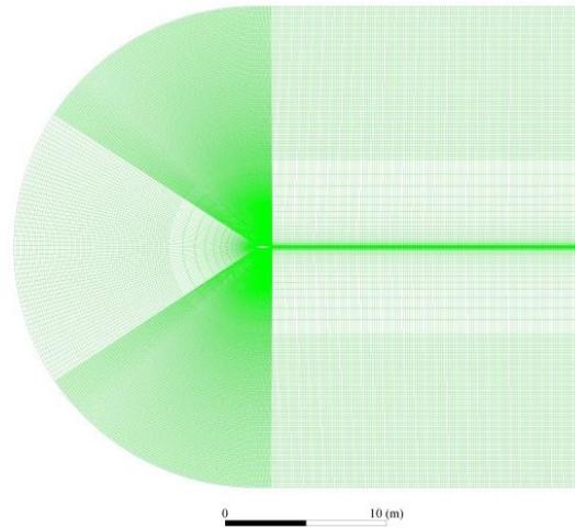
Fig. 5: Mesh of optimised airfoil
