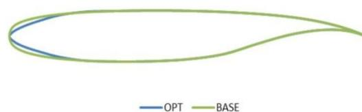
**Fig. 3: Whitcomb IL vs. optimized final airfoil**
