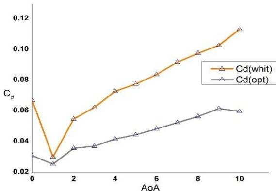
Fig. 9:  $C_d$  vs. AoA for Whitcomb IL and optimized airfoil
