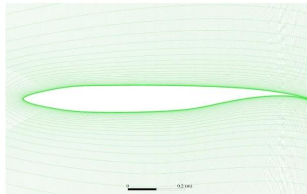
Fig. 6: Fine mesh around airfoil surface
