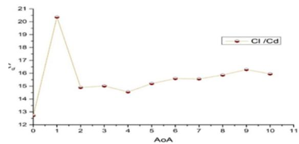
Fig. 10(a):  $C_l/C_d$  vs. AoA (Whitcomb IL airfoil)
