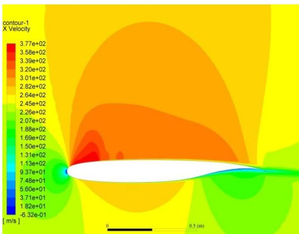
Fig. 13: Velocity field at  $M = 0.73$ ,  $AoA = 0^\circ$  - Whitcomb IL airfoil
