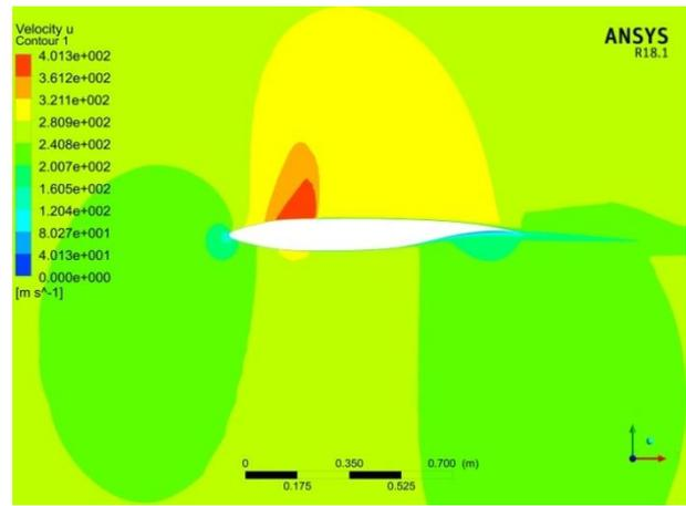
Fig. 14: Velocity field at  $M = 0.73$ ,  $AoA = 0^\circ$  - Optimized airfoil
