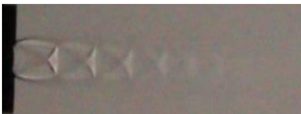
Fig. 9: Shadowgraph along uncontrolled jet at NPR5
