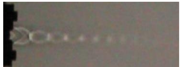
Fig. 15: Shadowgraph along elliptical perforated tabs at NPR5
