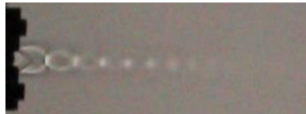
Fig. 12: Shadowgraph along elliptical solid tabs at NPR5
