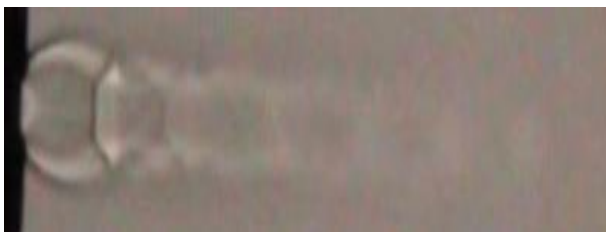
Fig. 8: Shadowgraph along uncontrolled jet at NPR8
